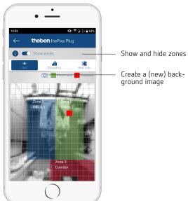
The motion/presence detected by the presence detector is displayed in green (motion) and red (presence).
