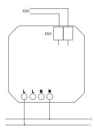
$oldsymbol{\Lambda}$  Secure device with an upstream type B or type C circuit breaker (EN 60898-1) with a maximum of 16 A.
