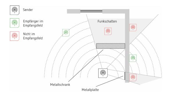
Radio shadow e.g. due to metal parts
