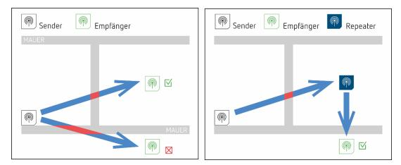
Wall or ceiling thickness effective for attenuation
