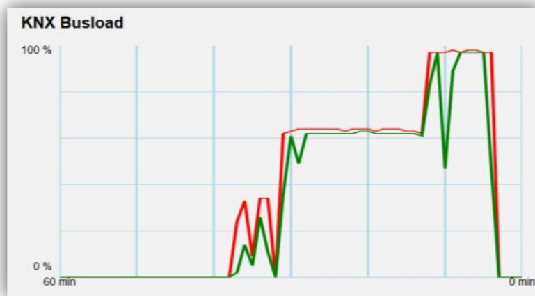
Figure 9 Interface web (charge du bus KNX)
