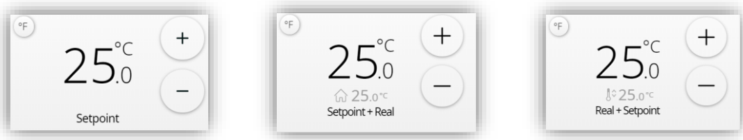
Figure 85. Setpoint Temperature with different indicator types
