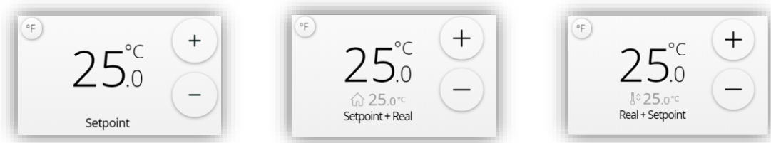
Figure 87. Setpoint Temperature with different indicator types
