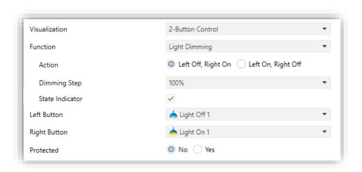
Figure 84 Light Dimming.
