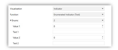
Figure 65 Enumerated Indicator (Text)
