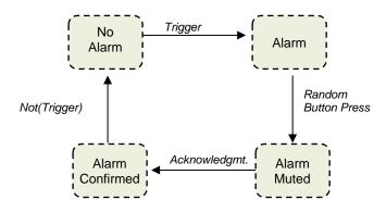
Figure 121 Alarm state diagram (case of confirmation previous to the alarm end)
