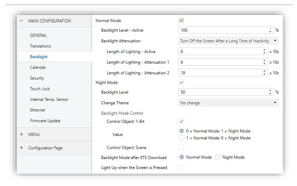
Figure 39 Backlight (Main Configuration)
