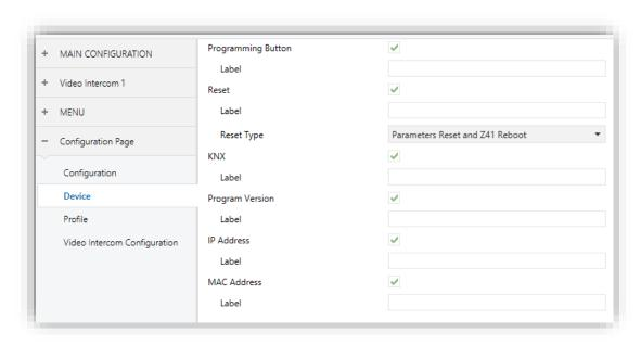
Figure 146 Device in Z41 COM (Configuration Page)
