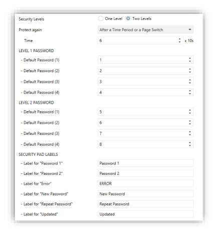
Figure 45 Security: Two Security Levels
