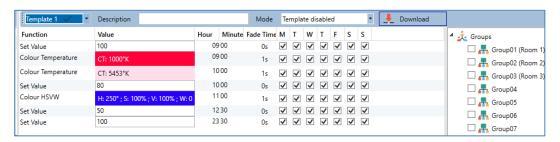
The middle part of the page is used to create an action list. All groups that have been selected, automatically perform an action at the configured time. Altogether a maximum of 300 actions can be stored on a DALI gateway if all templates are used. A context menu is available to control and create action lists.
