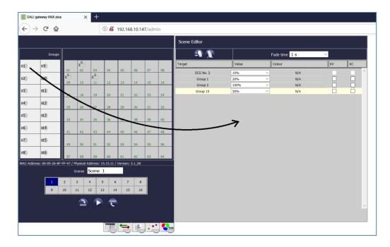
Please remember that only those ECGs can be used in a scene that have been defined as individual ECGs. If an ECG has been assigned, it can no longer be moved to the list. Once all elements have been dragged into the scene, the required values can be set.
