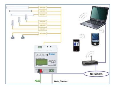
Use a standard patch cable to connect the device to a switch, hub or router of the IP network. You can also use a WLAN access point as network coupler. This means you can commission the DALI via a portable note book, tablet PC or mobile phone.
