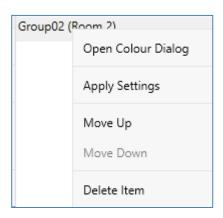
Connection to the DALI gateway KNX plus is required. The command is performed with the value and colour settings that have been defined for this group or ECG. This makes it possible to check properties before the whole effect is programmed. If "Keep value" or "Keep colour" have been set, the respective values will not be activated and the current value will be retained.
