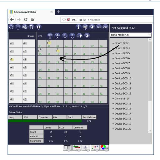
ECGs first appear as single ECGs and are therefore marked with an S (single). If you accidentally allocated them wrongly, simply remove them from their assigned ECG by clicking on
