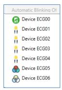
To identify the devices, switch the corresponding lamp on and off. If you select an ECG and press the right mouse button, a context menu appears from which you can select the required function.
