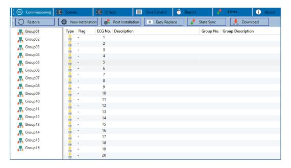
The group configuration is displayed in a tree structure on the left-hand side. The middle part shows a table for the ECG configuration and names. A list on the right-hand side shows the actual devices found in the system that have not yet been identified. During the planning phase the list is empty as the ETS is not yet connected to the system.
