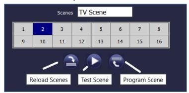
During programming you can assign a name (max. 10 characters) to the scene. Before saving the scene, enter the name in the text field above the scene block.
