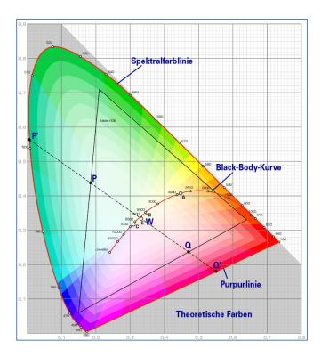
In devices that support the x-y coordinates method, the colour is set via two values between 0.0 and 1.0. However, because of the physical properties of an LED, even in an RGB LED module not every colour is practically possible. In practice, it is common to set the value which is closest.
