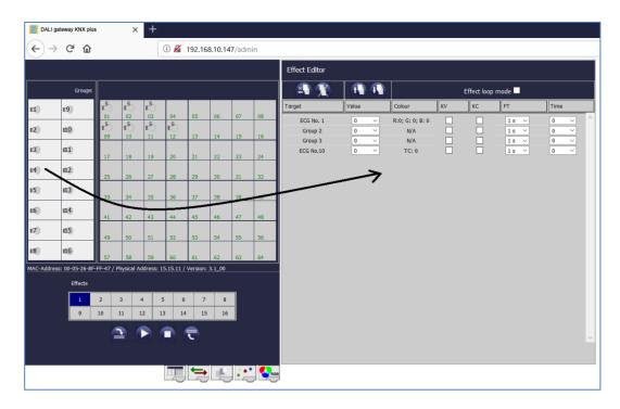
Please remember that only those ECGs that have been defined as individual ECGs can be used in an effect. An ECG that has been assigned to a group, can no longer be pulled into the list. Use the
