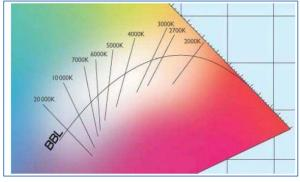
The points on this so-called black-body-line (BBL) are usually defined via a colour temperature in Kelvin. This makes it possible to exactly determine the white tone of a light between warm and cool with just one value. The colour temperature principle is therefore perfect for the control of white light fixtures (tunable white).
