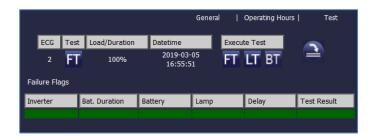
This display shows the type of test, test result and date and time of the last test. The status bar shows the error flags. A green bar means there were no error flags and the test was positive. A red bar signals a negative test result.
