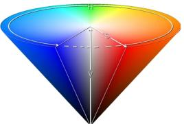
The value (V) is set via the value object number 41. Further objects are displayed for hue (H) and saturation (S). The hue is entered as a value between 0° and 360° and rotates around the colour circle making it easy to reach all colours of the circle.
