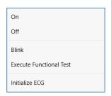
The context menu is also available at group level. During the identification process it might be useful to switch certain groups or all connected lamps on or off. You can also send broadcast commands via the context menu, in order to, for example, switch all lights on or off, see operation of DALI devices
