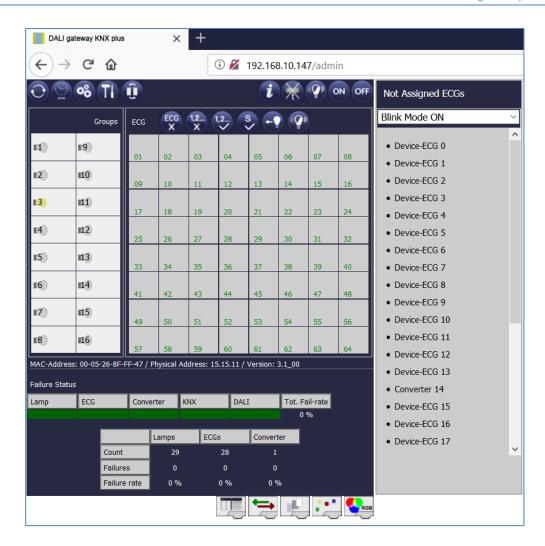
If you select an ECG on the right-hand side, it automatically changes to flashing mode in the standard setting (FLASH Mode ON). Once the device has been identified, use drag-and-drop to pull it to the previously planned ECG field in the middle.
