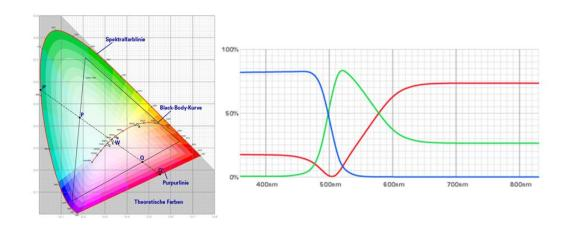
In the KNX the value range is converted to a range from 0 to 65535 (2 Byte integer). 65535 hence corresponds to the value 1 in the graphic.
