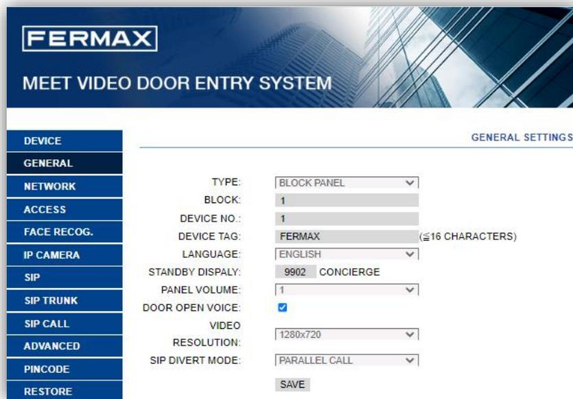
The screenshot displays the configuration interface for the FERMAX MEET VIDEO DOOR ENTRY SYSTEM. The interface is titled 'FERMAX MEET VIDEO DOOR ENTRY SYSTEM' and 'GENERAL SETTINGS'. On the left, there is a navigation menu with the following items: DEVICE, GENERAL (selected), NETWORK, ACCESS, FACE RECOG., IP CAMERA, SIP, SIP TRUNK, SIP CALL, ADVANCED, PINCODE, and RESTORE. The main configuration area includes the following fields:
