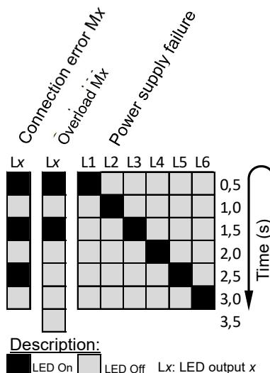
Figure 2: Error notification through grille status LED
