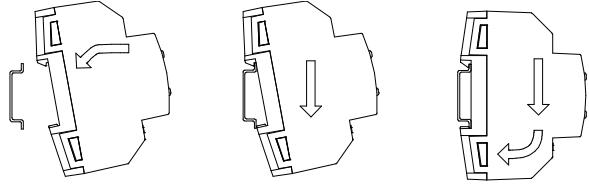
Removing ZoningBOX 6 from DIN rail:
