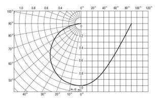
Figure 3: Lighting level sensor sensitivity
